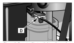
Figure 2: Do not adjust or tighten the engine governor screw.
